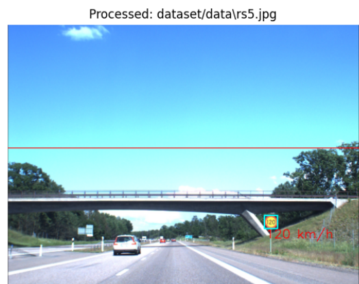
Fig. 10. False detection of the Hough Transform
