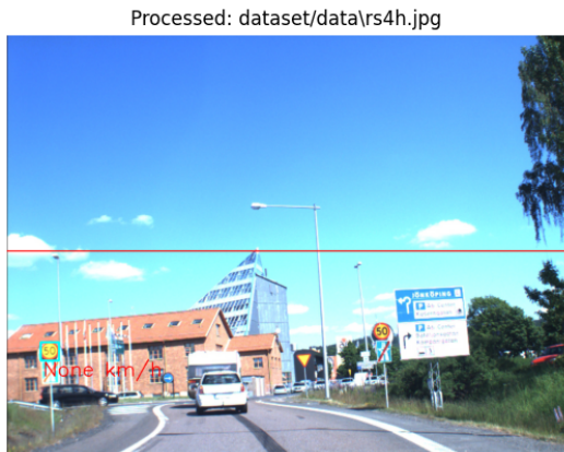
Fig. 11. Erroneous detection from the OCR module, and no detection from the Hough transform on the right side
