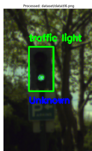
Fig. 7. Erroneous detection due to large ROI
