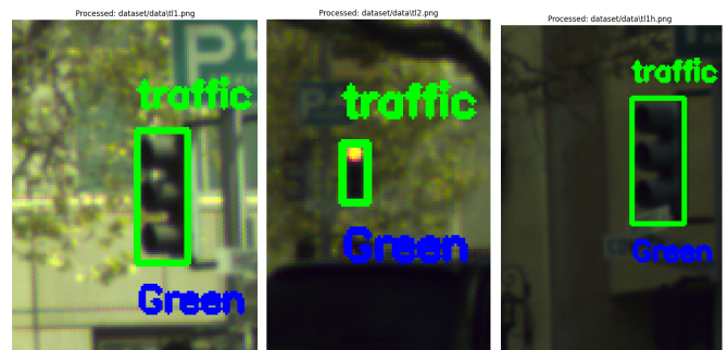
Fig. 6. Erroneous detection due to background tonality
