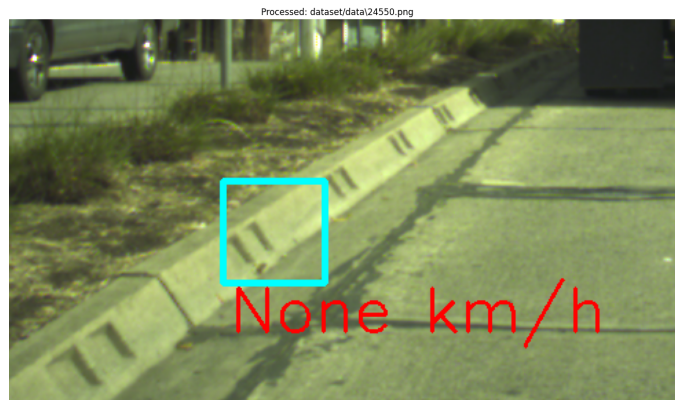
Fig. 8. False detection of the Hough Transform
