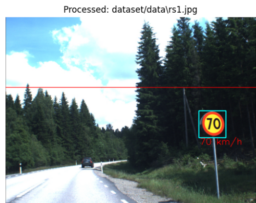
Fig. 9. False detection of the Hough Transform
