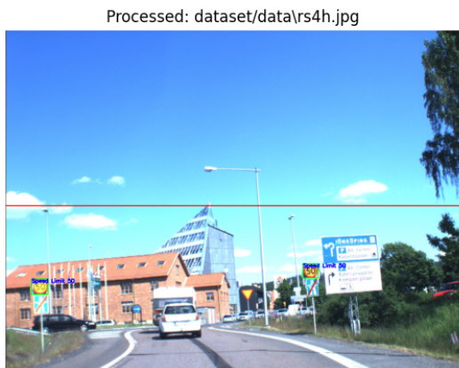
Fig. 3. Custom trained YOLO detection of difficult road sign
